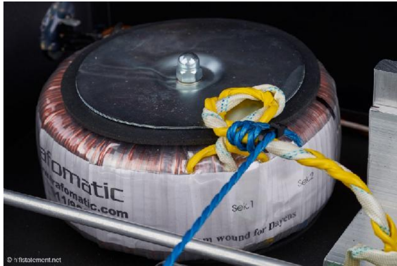
The stately transformer is not mass-produced but specially manufactured
